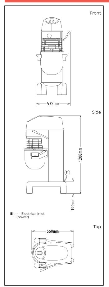
Electric Supply voltage: 200-240 V/1N ph/50/60 Hz Electrical power, max: 1.1 kW **Total Watts:** 1.1 kW Capacity: Performance (up to): 7 kg/Cycle Capacity: 30 litres Key Information: External dimensions, Width: 532 mm External dimensions, 685 mm Depth: External dimensions, Height: 1208 mm **Shipping weight:** 106 kg **Cold water paste:** 7 kg with Spiral hook **Egg whites:** 50 with Whisk
